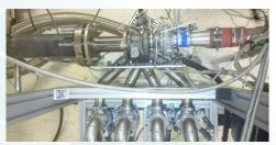
The objective is to test turbochargers in a more realistic environment than with a traditionnal bench, thanks to the use of a specific test bench.
